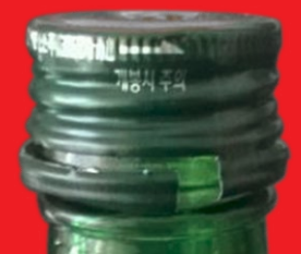
Demolition of safety ring
