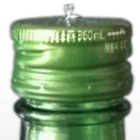
Incomplete threaded flange
