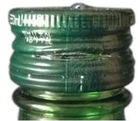
Burst open safety ring
